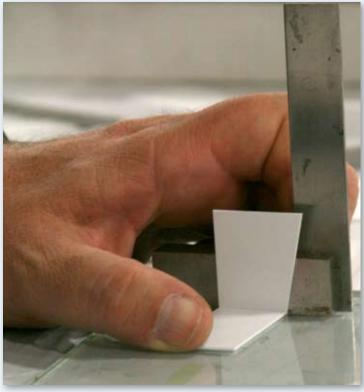
▲ **Step 3:** When assembling your structure, attach the back and sides first. When attaching the pieces, use a square to help form a square joint.
