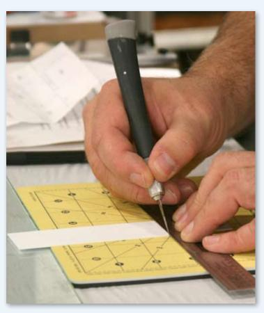
▲ Step 1: Cut the sides and base of the structure to size. Cut on the back side of the piece in case the knife slips, that way the good side will not be marred. When cutting through styrene, make several light passes over the piece rather than forcing your blade through the styrene in one cut.
