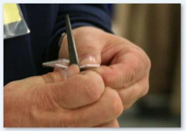
▲ Step 7: When creating the doors for a structure, scrap pieces of styrene may come in handy as you may already have a piece that is close to the dimensions you need. After cutting the door to shape, compare the door with the opening to make sure they are the same size. If needed, file the opening to fit the door.
